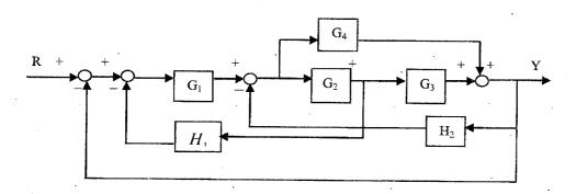
[c] Determine the transfer function using signal flow graph.
